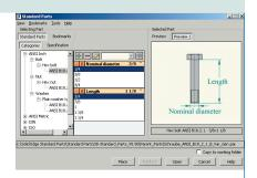
benefits of 3D virtual prototyping. Solid Edge Standard Parts makes component libraries easily accessible, so users can quickly find the right part and effortlessly place them in Solid Edge assemblies, all within company standards.
