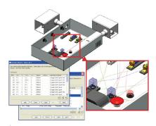
can quickly establish a "rats nest" of wires from a predefined connector on one component to a corresponding connector on another.
